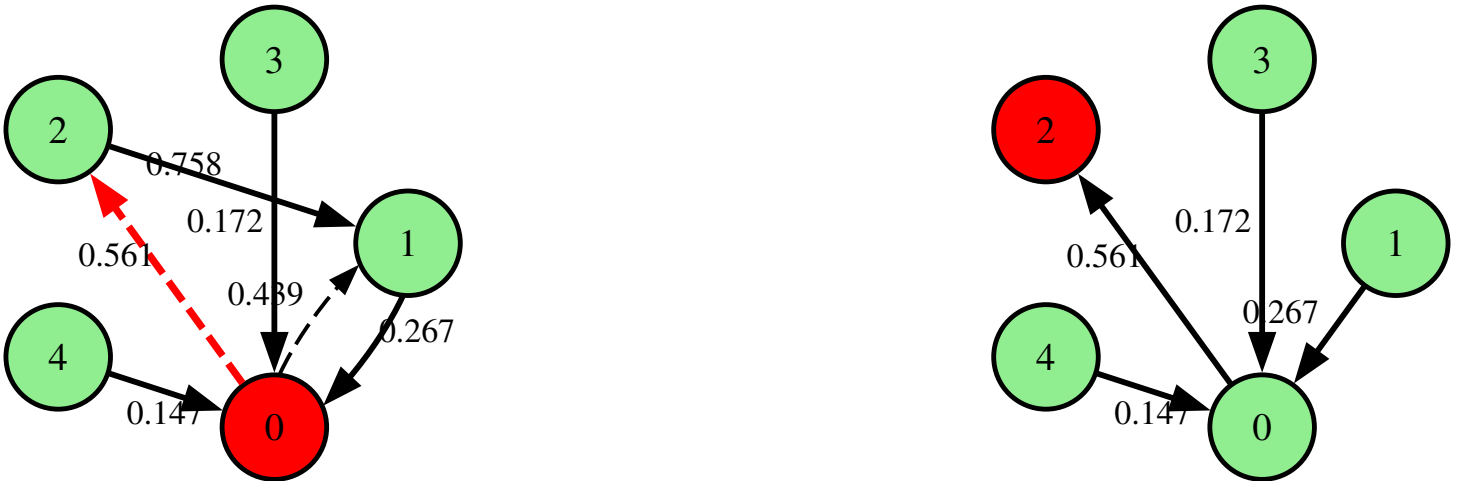
Figure 4: The Markov chain on \Theta works as follows. When the state is the in-arborescence \theta on the left, we can select each arrow outgoing from the root 0 with probability given by the original Markov chain (dashed edges). Say we select the arrow (0, 2) (red dashed edge). Then we add this arrow and remove the one outgoing from 2. The result is the in-arborescence on the right.
